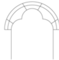
Unequal round arch or Rampant round arch
