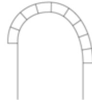
Unequal round arch or Rampant round arch
